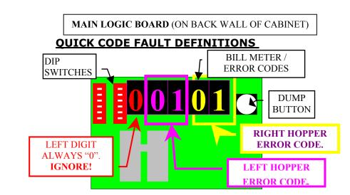
Press the "DUMP" Button before turning off changer. Match the code to samples below to find out why the hopper(s) were shut down.
